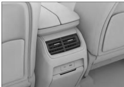
Adjust the direction of airflow by moving the button in the middle of the outlet.
