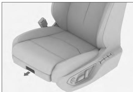
Pull forward and hold the clasp on the lower part of the seat cushion to pull out the front end of the seat cushion or push it back.
