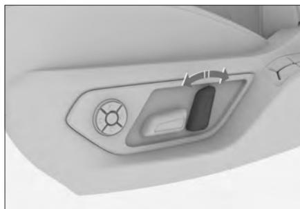
Toggle the top of the button back and forth to adjust the angle of the seat back.
