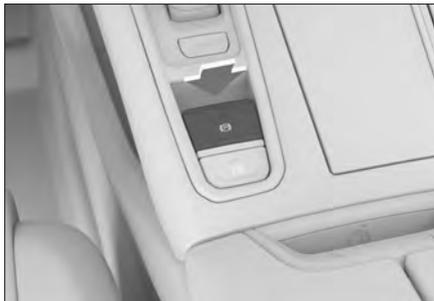
With the power switched ON, step down the brake pedal and press down on the EPB switch to release the parking brake. The parking brake indicator light (Ⓢ) on the combined instrument panel will go out.
