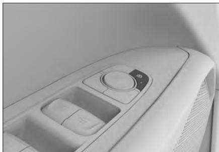
The central button is located on the front-row door armrests. Make sure all the doors are shut securely, then press the central button to lock or unlock all the doors.
