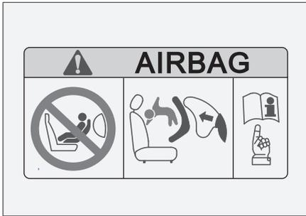
This label is located on the front passenger's sun visor. It is to remind you that this car is equipped with front airbags. Make sure to read the relevant notes.
