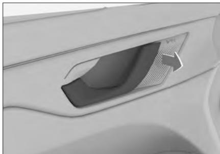
Pulling on the inside door handle will unlock a locked door. Pulling on it again will open the door.
