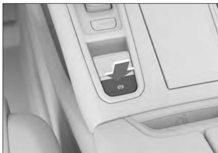
When the vehicle is on a slope, at a red light or in stop-and-go traffic, automatic vehicle hold (AVH) frees the driver from having to keep the brake pedal pushed down for an extended period of time or having to engage the electric parking brake frequently. This makes driving more comfortable for the driver and lowers the risk of the vehicle rolling.
