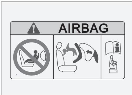
This sticker is located on the front passenger side sun visor to remind you that your vehicle is equipped with a front airbag. Please note the related matters.
