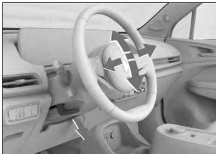
1. Release the adjustment lever under the steering wheel.
