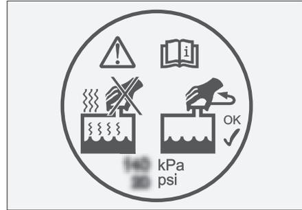
This label is located on the warm air overflow tank, and is to remind you not to open the overflow tank cover while the warm air system is on or has not cooled completely. Otherwise, hot liquid and steam expelled under pressure could cause burns.
