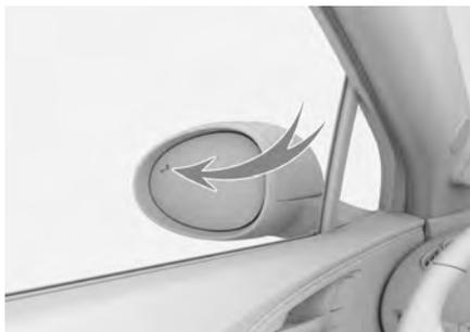
The warning lights are on the surface of the left and right side mirrors.
