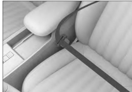
3. Pull the shoulder belt upwards, and adjust the waist belt to ensure a snug fit. This will reduce the possibility of injury to the pelvis in a collision.
