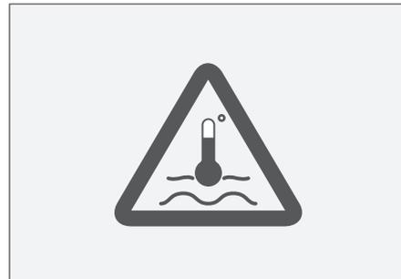
This label is located on the powertrain system coolant overflow tank; its purpose is to remind you not to open the overflow tank cover when the drive motor is too hot. Otherwise, hot liquid and steam expelled under pressure could
