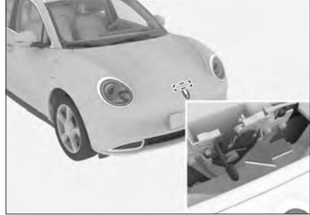
3. Unhook the support rod and insert the front-end into the slot in the bonnet to hold it open.
