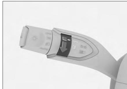
When low-beam is on, twisting the fog lamp switch to  $\text{0}$  the rear fog lamp position turns the rear fog lamp on or off. When you release the knob it will go back to its original position.
