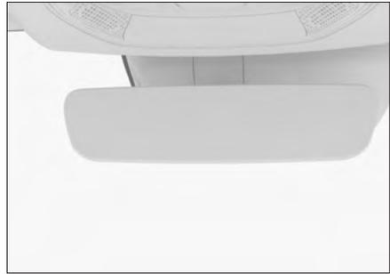
The rear view mirror automatically reduces glare according to the intensity of the headlamps of vehicles behind you.
